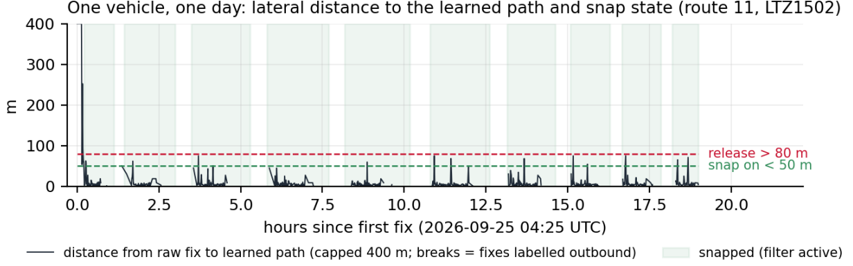
Figure 11: Route 11, vehicle LTZ1502, 2026-09-25: distance from each raw fix to the learned inbound path, and the periods the filter was engaged. Breaks in the line are trips labelled outbound, which snap to the other path.
